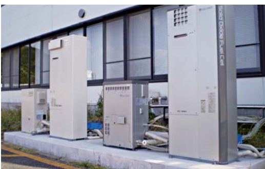
Photo: Laboratory test of Solid Oxide Fuel Cell (SOFC)
